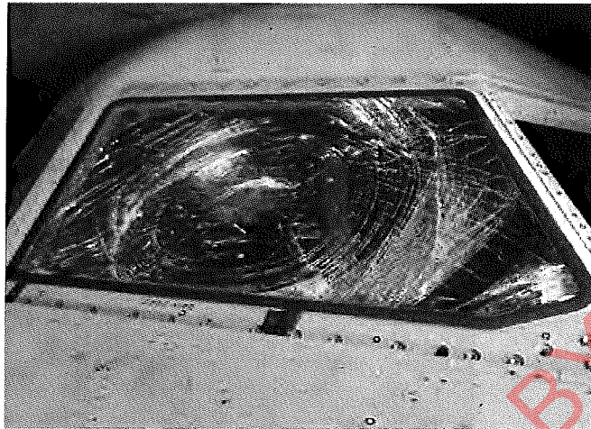
Figure 7-10: Photograph of windshield damage for [REDACTED]
