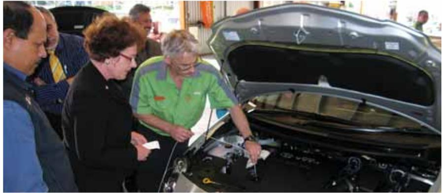
ASSOCIATE TRANSPORT MINISTER, JUDITH TIZARD (PICTURED) WATCHING AS THE TEMPERATURE PROBE IS INSERTED INTO THE OIL IN THE ENGINE TO MAKE CERTAIN THE ENGINE IS THE RIGHT TEMPERATURE FOR THE TEST TO BE PERFORMED.
